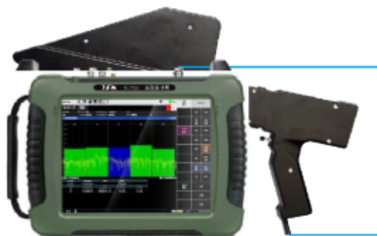
Figure 7.1 Schematic connection of hand-held DF antenna with RMT series spectrometer
