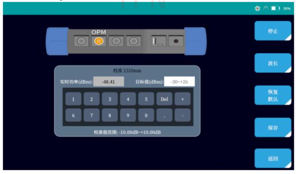
The optical power meter supports user self-calibration, and the calibration deviation range does not exceed ±10dB.
