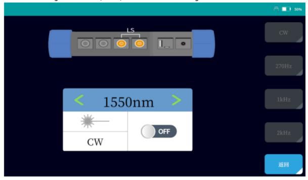
Step 1: Connect the LS interface (consistent with the OTDR interface);
